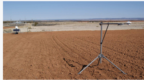
Fig. 4: Example of a proper installation of an albedometer (prospection phase). Image credit & Copyright: GroundWork Renewables, Inc.
