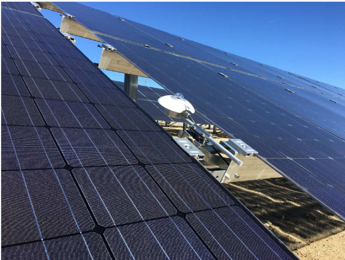
Fig. 5: Example of a tilted installation of an albedometer (operation phase). Image credit & Copyright: GroundWork Renewables, Inc.
